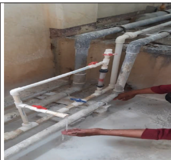
Calibration of Rotameter for chlorine dosing system at Bode Water Treatment Plant
